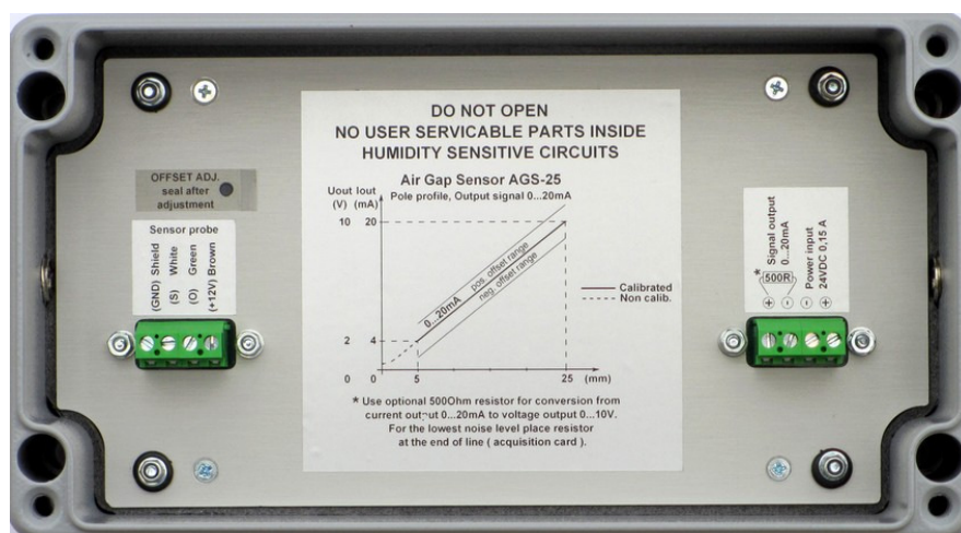
Figure 10d. AGS Signal Conditioner unit enclosure with cable inlets (CAB) (after S/N 144701)
