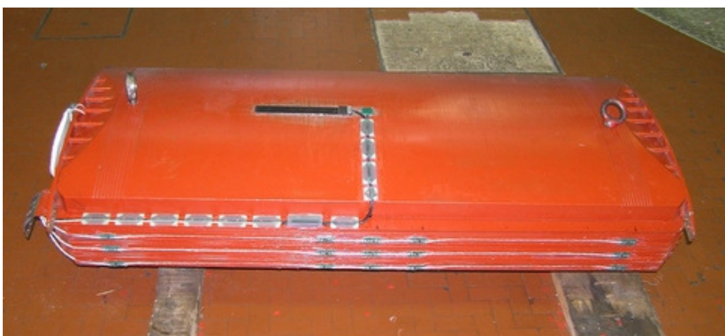
Figure 13. AGSP sensor probe installed at rotor pole (AGSP sensor pictured next to Magnetic field sensor in the middle of rotor pole)
